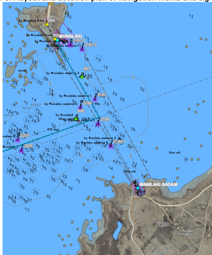
Munalaiu-Manilaiu Harbour Port layout and Location plan of navigation marks and signs
